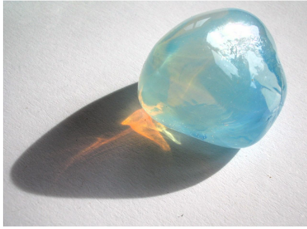
Figure 2: Rayleigh scattering in opalescent glass 32
